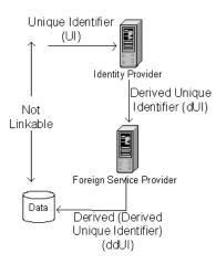
Figure 3: Depicting the process to eliminate cross linking using unique identifier
