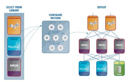
*Figure 1. Example cloud-based deployment of an application onto a two-tier Web server architectural pattern.*
