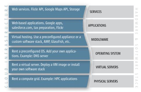
Figure 6. Cloud computing means using IT infrastructure as a service — and that service may be anything from renting raw hardware to using third-party APIs.
